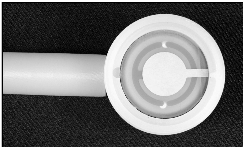
Figure 8. QCM Crystal in Crystal Holder cavity with wrap around electrode pointing towards reference pin.
